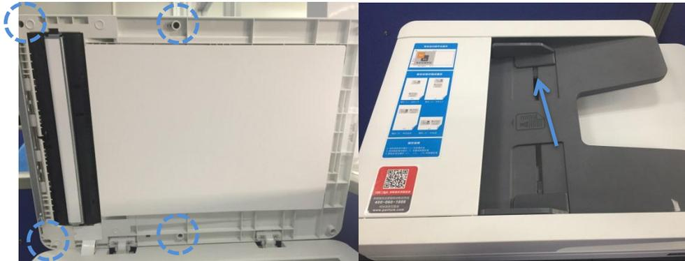
2. Remove four sheet metal screws, sheet metal assembly and then ADF motor.
