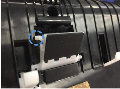
2. Open the upper ADF cover, take the paper-feeding assembly from the area between two baffles, remove the snap spring and gear shaft, and pull out the bearing buckle and bearing.
