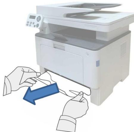
3. After pulling out the jammed paper, install the paper tray into the printer, and close the front cover. The printer will automatically recover printing.
