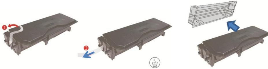
5. Install the drum component along the inner track to finish installing toner cartridge.
