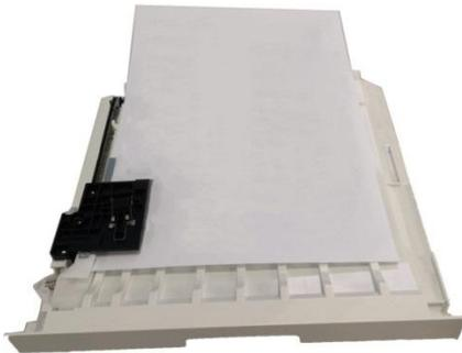
3. If the jammed paper is not taken out with the duplex printing unit, open the paper tray and directly take out the jammed paper from the bottom.
