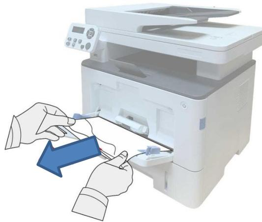
2. After removing the jammed paper, reload paper into the multi-purpose tray; press the front cover button to open and close the front cover, and the printer will resume printing..
