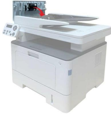
4. If it is difficult to remove the jammed paper, try opening the scanner cover and removing the jammed paper from the pressing plate.
