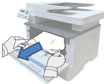
7. After taking out papers jammed, install the laser toner cartridge again and close the front cover, then the printer will recover printing.
