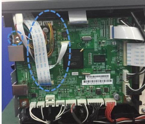
2. Remove two screws of the hinge support rod and then the hinge support rod (hold the scanner assembly by hand).
