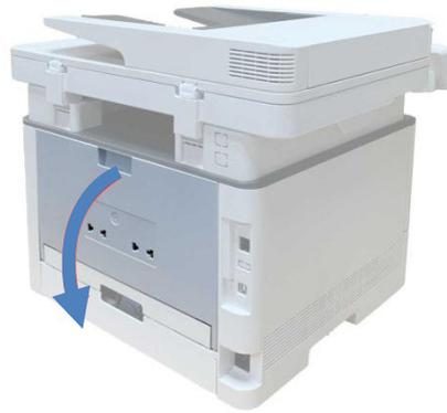
3. Open the fuser door using the handles on both sides.
