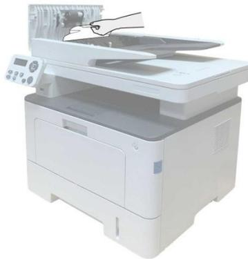
3. After removing the paper jammed, close the top cover and then the printer will be back to the ready state.
