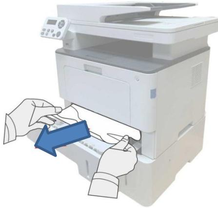
3. After removing the jammed paper, reinsert the automatic tray into the printer, and the printer will resume printing automatically.
