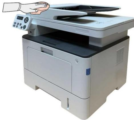
3. Lift the scanner cover and gently wipe the glass platen with soft cloth.
