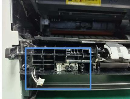
2. Release the screws and remove the sensor substrate. (Pay attention to raise the detector handle when you remove the sensor substrate, in case the sensor handle is damaged.)
