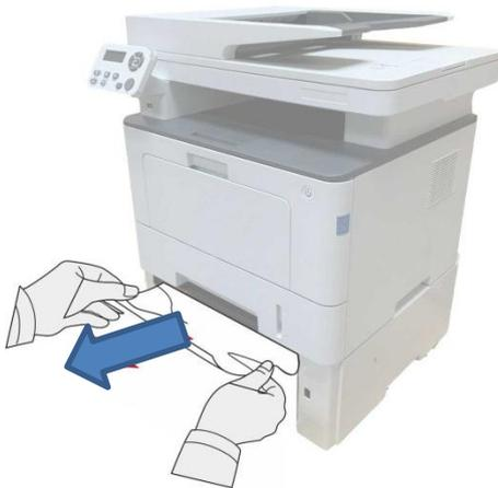
3. After removing the jammed paper, reinsert the optional tray into the printer, and the printer will resume printing automatically.
