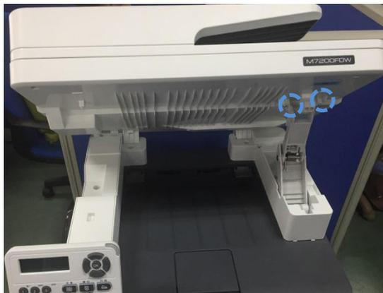
3. Hold the scanner/ADF assembly by hand, remove three screws of the upper side cover, and pry out the upper side cover with the slotted screwdriver.
